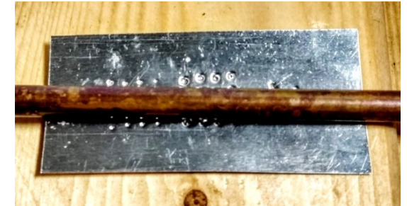
Rolling the sheet to flatten it
