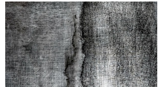
Aluminium sheet with streaks
